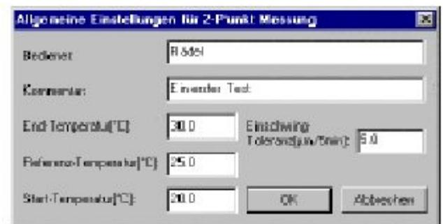
At the two point measurement method a third temperature point is used. That means the average thermal expansion for a low temperature range and for a high temperature range is calculated by a selectable reference temperature. The result for each sample will be stored in an ASCII (text) file.
